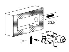
Step3: Install the tap body to the right position and make sure Hot&Cold water inlets
