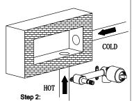
Drill the holes on the wall and connect the cold water inlet and hot water inlet to proper positions.
