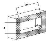
Step1: Determine the fixing position for the faucet body. Make a groove in the wall according to the faucet body. The dimension of the groove should be 200mm x55mm.
