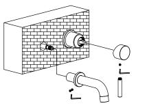
Screw off the handle lever, and assemble the handle and spout using the Allen key. Then fix the handle
